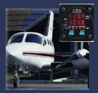
Accurate, instantaneous fuel flow rate and consumption data with cockpit display integration. Built for high reliability with stainless steel construction, meeting fire resistance standards.
